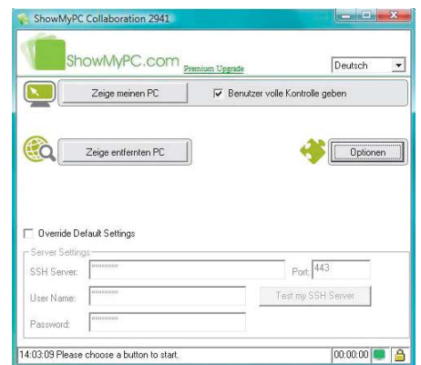
Displaying Windows desktop is shown over a built-in VNC server in ShowMyPC, which is unsuccessful at Vista's UAC dialogues.
